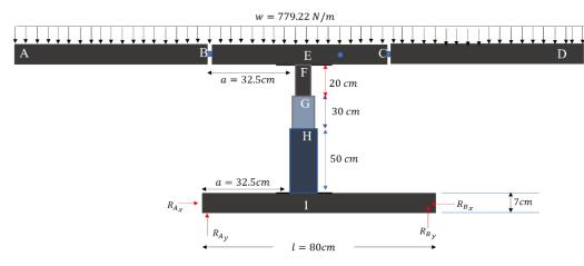
Figure 9. FBD of the design as a whole system in the sleeping position.
