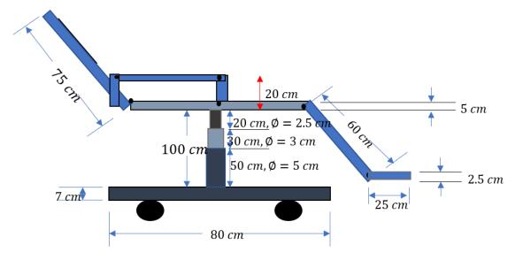
Figure 2. Two dimensional drawing of the chair.
