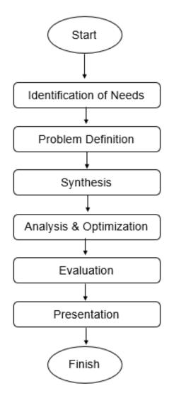
Figure 1. Stages of mechanical design
