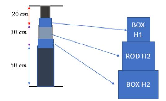
Figure 7. Schematic of the leg support by employing the hydraulic system as the adjustable height.
