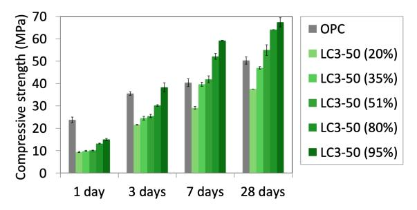
Figure 8. Compressive strength of LC<sup>3</sup>.
