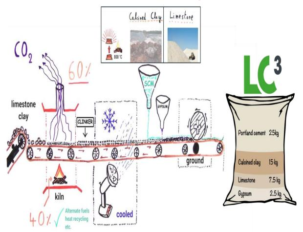
Figure 1. Illustration of LC<sup>3</sup> production.
