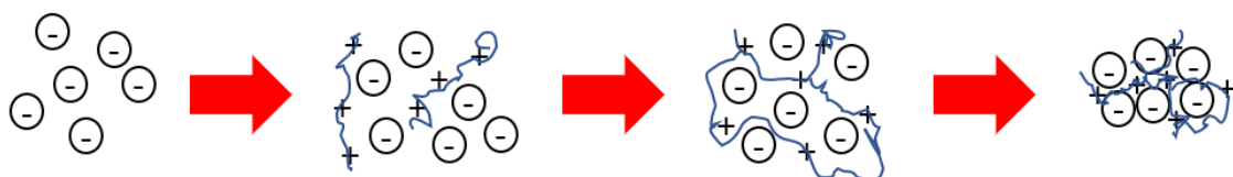
Figure 5. Schematic diagram of bridging mechanism.
