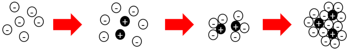
Figure 3. Schematic diagram of charge neutralization.
