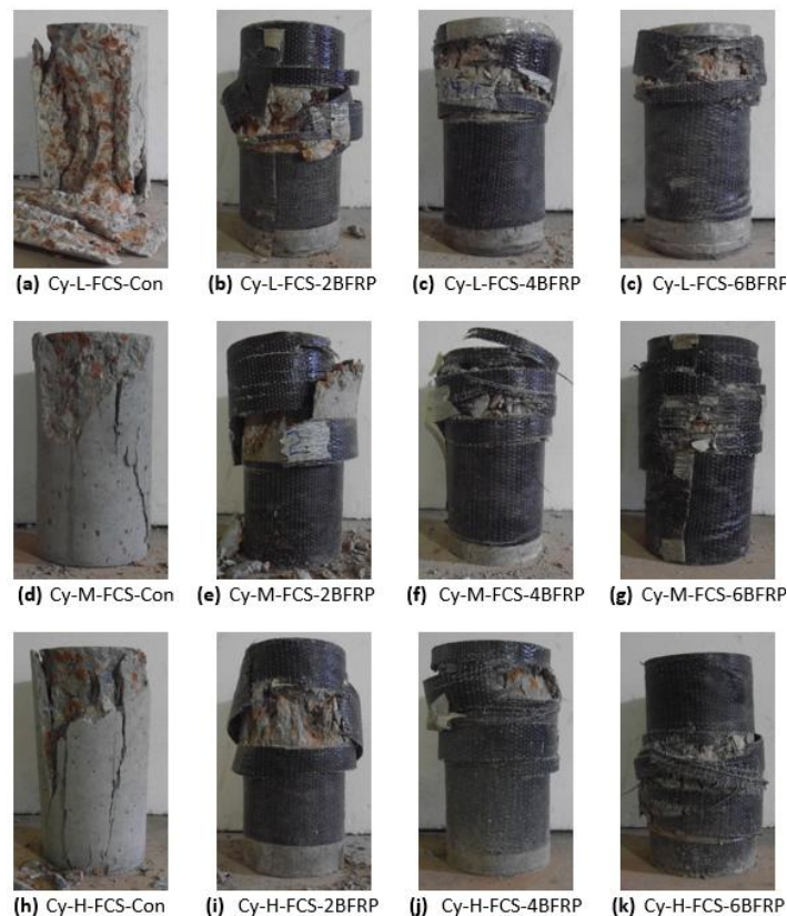
Figure 4. Failure modes of Group 1 specimens: (a) Cy-L-FCS-Con; (b) Cy-L-FCS-2BFRP; (c) Cy-L-FCS-4BFRP; (d) Cy-L-FCS-6BFRP; (e) Cy-M-FCS-Con; (f) Cy-M-FCS-2BFRP; (g) Cy-M-FCS-4BFRP; (h) Cy-H-FCS-Con; (i) Cy-H-FCS-2BFRP; (j) Cy-H-FCS-4BFRP; and (k) Cy-H-FCS-6BFRP.
