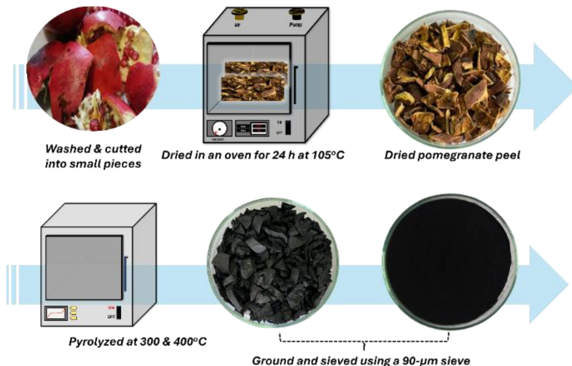
Figure 1. Process sequence for producing powdered biochar from pomegranate peel.
