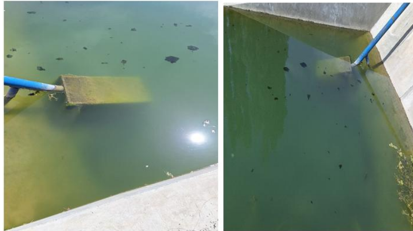
Figure 5. The water purification filter is installed in the pond in a polluted condition.
