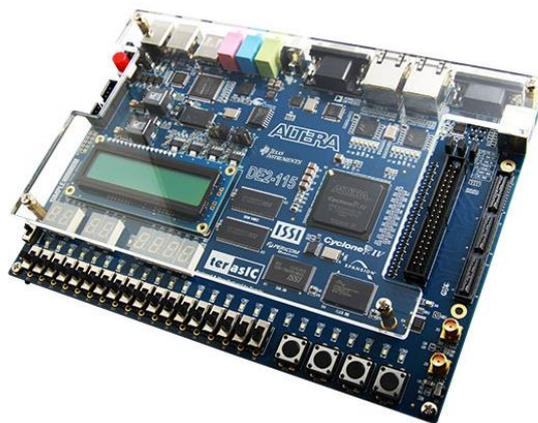
**Figure 28.** Terasic Altera DE2-115 Cyclone IV EP4CE115F29C7N
