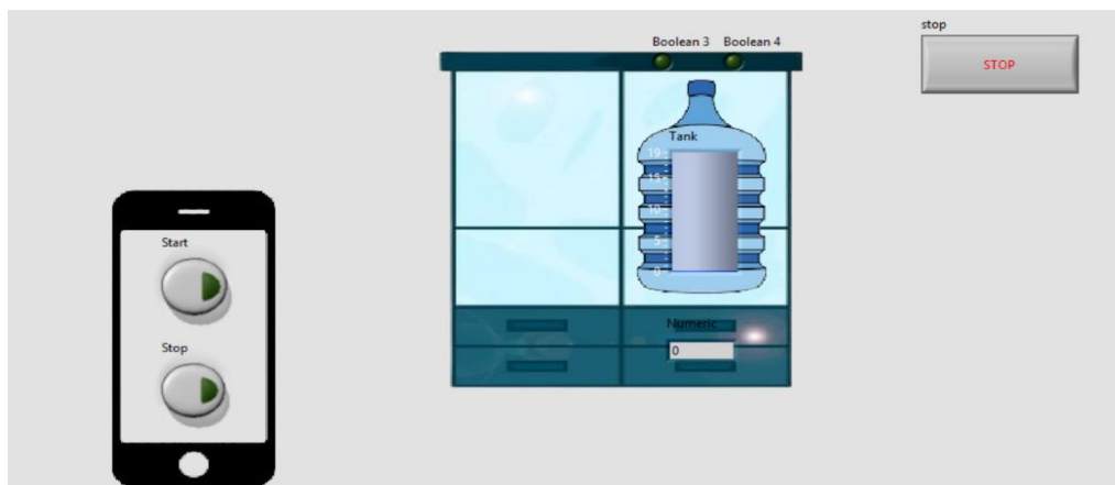
Figure 9. Front panel design of the automatic water gallon filling control system
