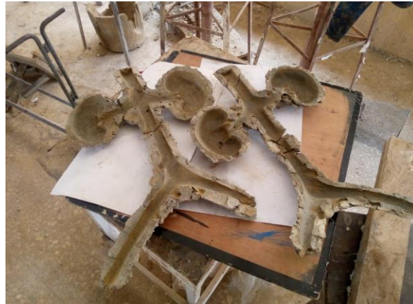
Figure 1. Casted mold (right and left side).
