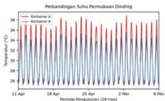
(6c) Comparison of the surface temperature of the walls in the container A&B (°C)
