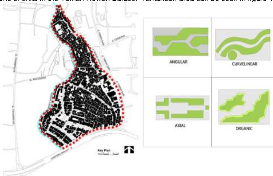
Figure 11. Void and Solid as Space Unit in Balubur Tamansari Area Source: Personal archive, 2014-2018; Trancik, 1986
