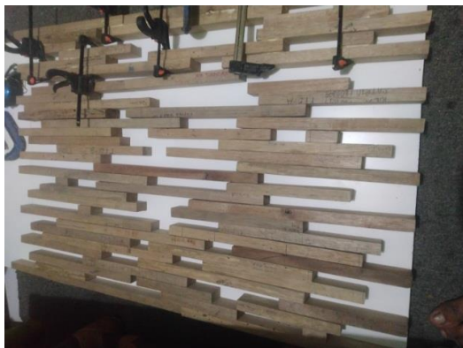
Picture 7. Arranging the woods with glued and clamped
