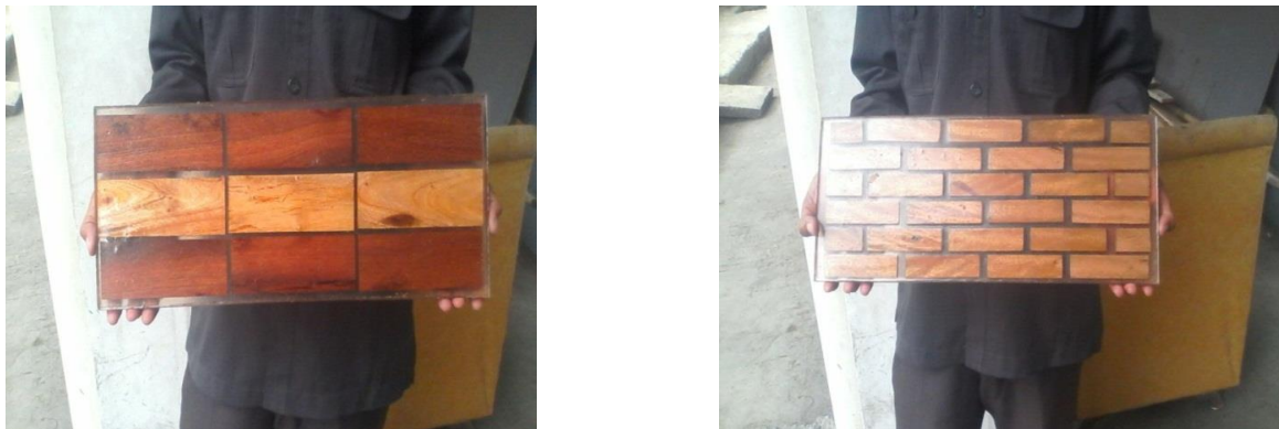
Picture 2. The last result of wood waste artificial board and resin.
