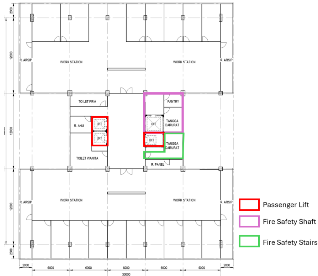
Figure 2. Existing conditions of fire man access and fire safety exit (Source: Author, 2025)
