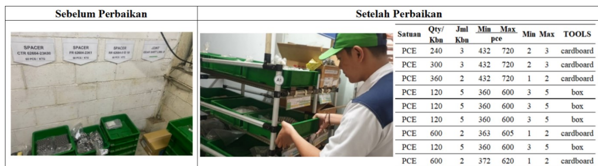
Figure 2. 6 Results of Improvement from Min-max Stock and Shutter Rack Implementation.
