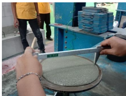
Figure 1. Mortar Flow Test
