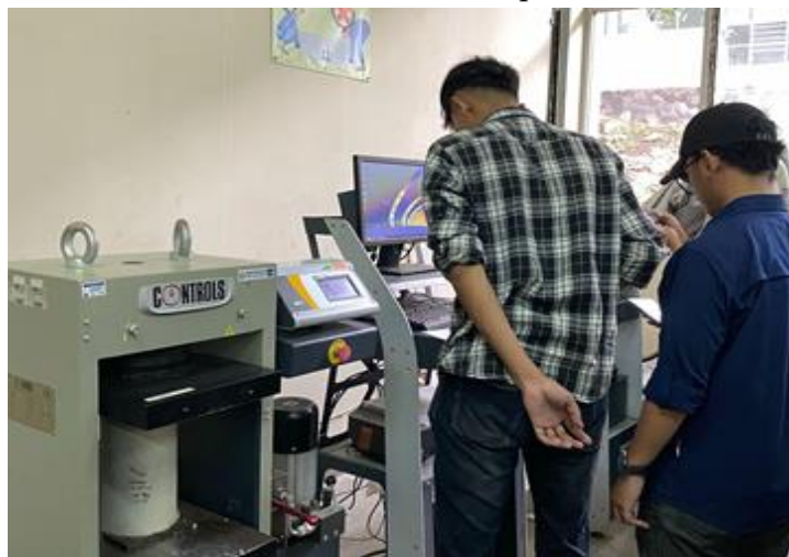
Figure 6. Concrete Compressive Strength Test
