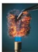
Steel wool heated in air (about 20% O 2 ) glows red-hot but oxidizes to Fe 2 O 3 slowly
