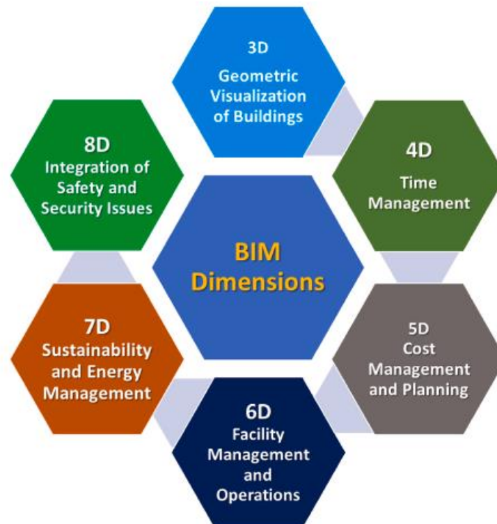
Figure 2. BIM Dimensions (Source: Biswas HK, Sim TY, Lau SL. Impact of Building Information Modeling and Advanced Technologies in the AEC Industry: A Contemporary Review and Future Directions. Journal of Building Engineering . 2024)
