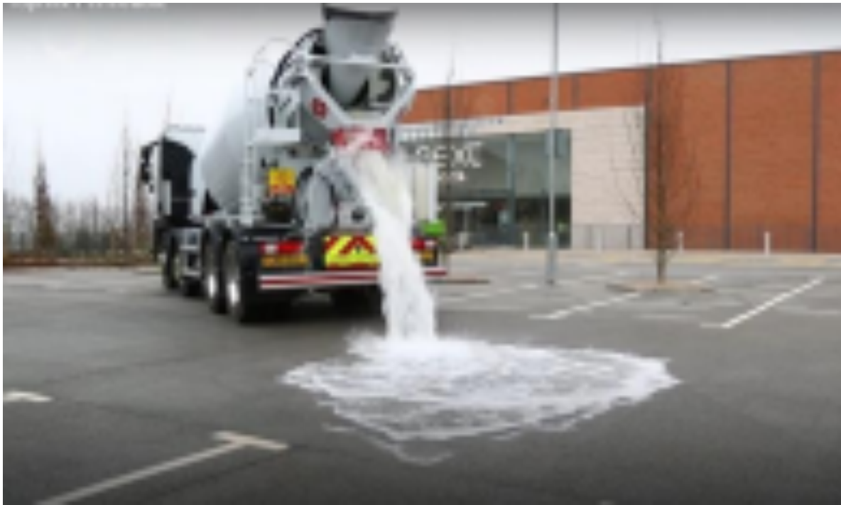
Figure 4. Asphalt Infiltration Capability Experiment.
