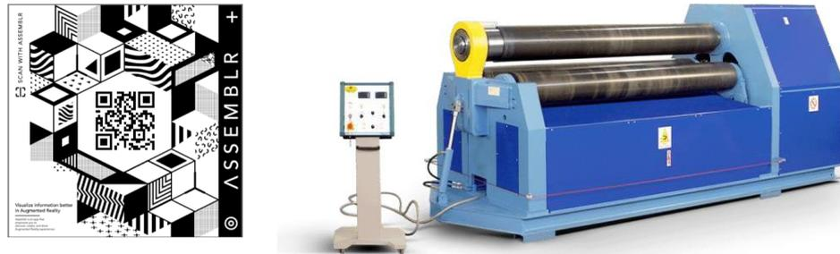
**Gambar 2.** Roll Bending
