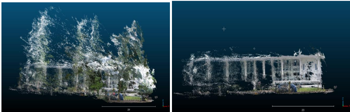
Figure 16. Action video camera point cloud results before (left) and after (right) filtering process
