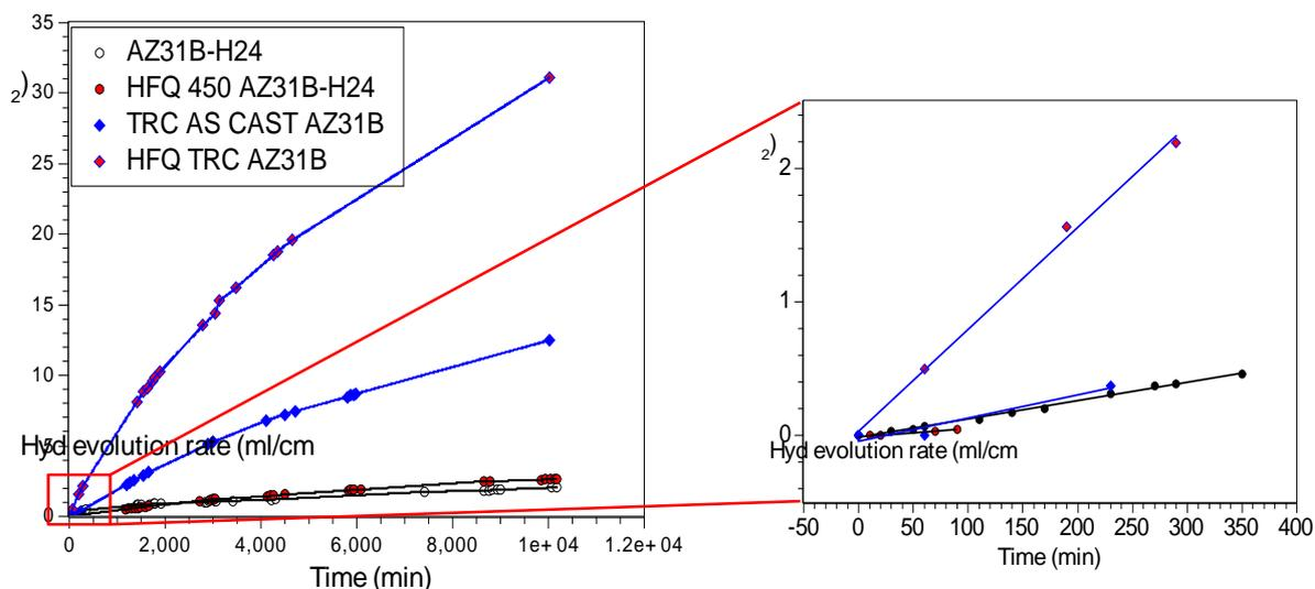
Figure 4. (a) Hydrogen evolution rate of alloys for 7 days (168 hr) and (b) Hydrogen rate during early duration ~5 hours.
