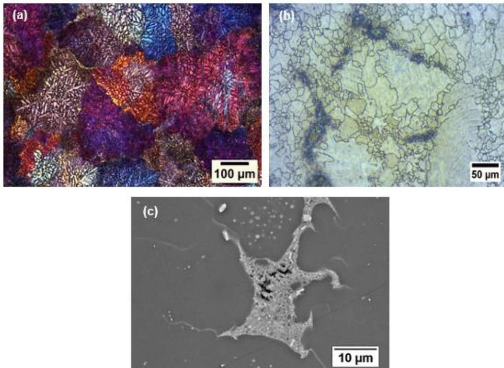
**Figure 3.** The microstructures of: (a) AZ31B twin roll cast (TRC) with fully dendritic structure and (b) HFQ AZ31B twin roll cast, showing equiaxed grain with (c)  $\beta$ -Mg<sub>17</sub>(Al, Zn)<sub>12</sub> particle.
