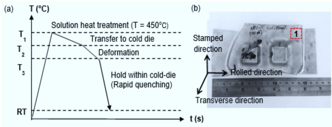
**Figure 1.** (a) Schematic diagram illustrating the HFQ process and (b) optical image of HFQ TRC AZ31B magnesium alloy sheet. The square labelled as 1 indicates the area for microstructure and corrosion characterisation
