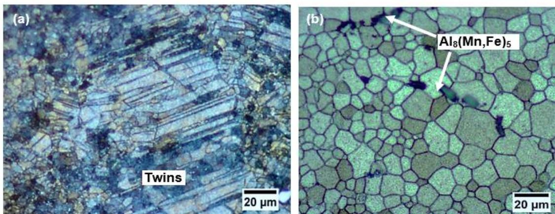
**Figure 2.** Optical images of: (a) as-received AZ31B-H24 Mg wrought alloy; (b) HFQ AZ31B-H24 sheet with bimodal distribution of  $\text{Al}_8(\text{Mn,Fe})_5$  particles.
