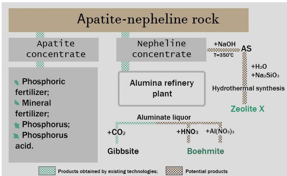
**Figure 1.** General scheme for obtaining potential products from nepheline raw materials.
