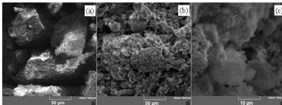
**Figure 4.** Electron microscope images (a) - raw nepheline concentrate; (b) and (c) - nepheline concentrate after activation in the presence of sodium hydroxide.
