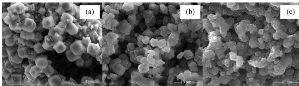
**Figure 7.** SEM samples: (a) – zeolite obtained after hydrothermal synthesis of activated kaolin clay: synthesis time 3 hours, synthesis temperature 95 °C; (b) – zeolite obtained on the basis of crushed nepheline concentrate: synthesis time 24 hours, synthesis temperature 95 °C; (c) zeolite derived from bauxite (Belviso, 2013).
