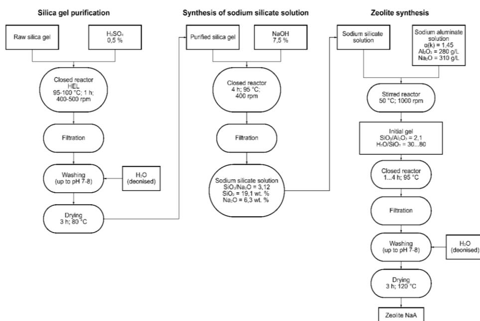
**Figure 2.** Scheme for obtaining zeolite from silica gel.
