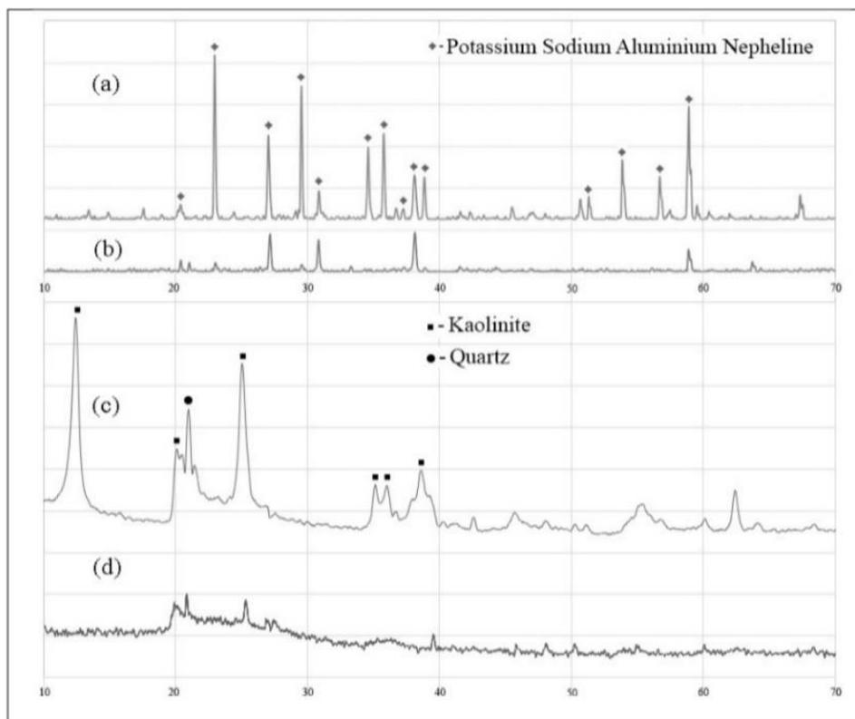
**Figure 3.** XRD: (a) - original nepheline concentrate without activation; (b) - nepheline concentrate after thermal activation in the presence of sodium hydroxide; (c) - kaolin clay prior to activation in the presence of sodium hydroxide, (d) – kaolin clay after thermal activation in the presence of alkali.
