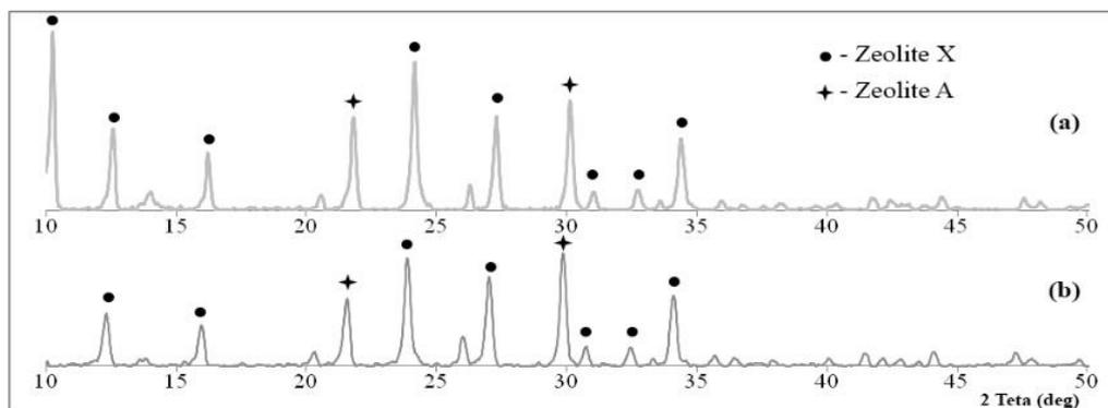
**Figure 6.** XRD of zeolites derived from kaolin clay.
