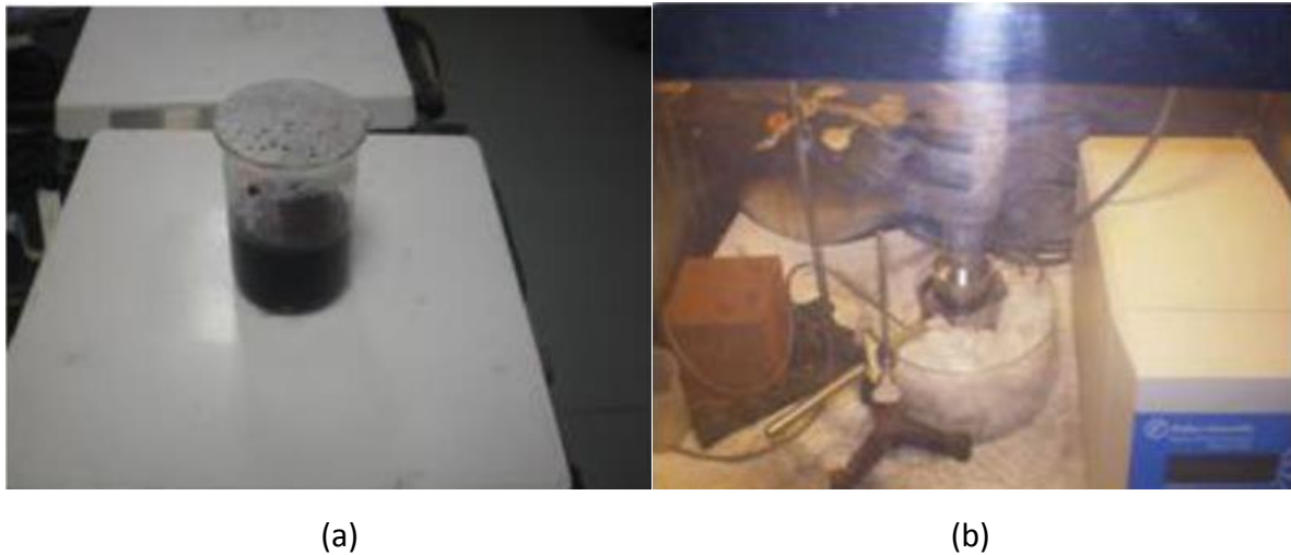
Figure 2. Dispersion equipment: (a) Magnetic Stirrer and (b) Sonication horn
