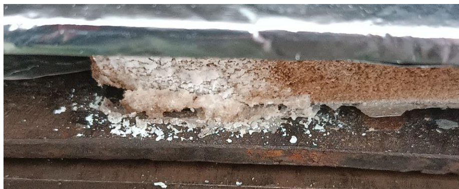
Figure 4. Lamina that treated with borax when compressed.
