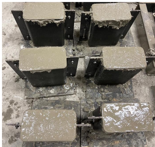
Figure 6. Construction of specimens.
