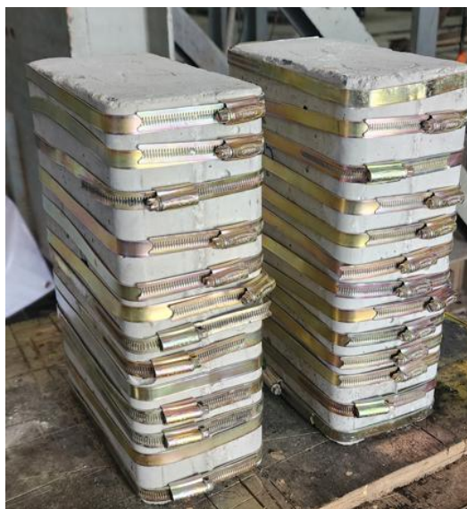
Figure 7. Typical low-cost steel clamp confined specimens.
