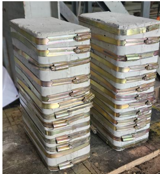
Figure 7. Typical low-cost steel clamp confined specimens.
