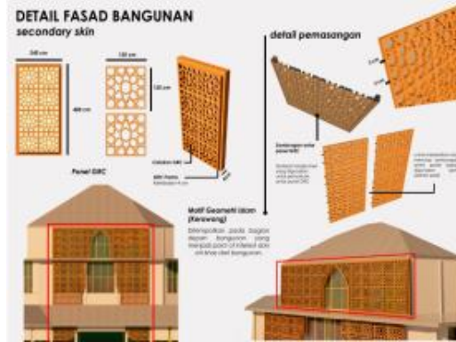
Figure 6. Placement and design of GRC applied in Islamic Fashion Institute facades (Source: Amalia S, 2020)
