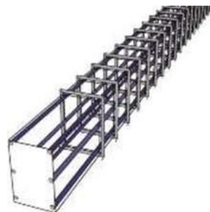
Gambar 23, Balok beton bertulang
