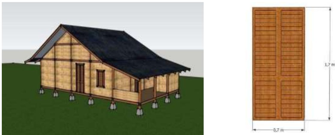
Figure 23. Door Openings in the Sulah Nyanda House (Source: Personal Document, 2024)
