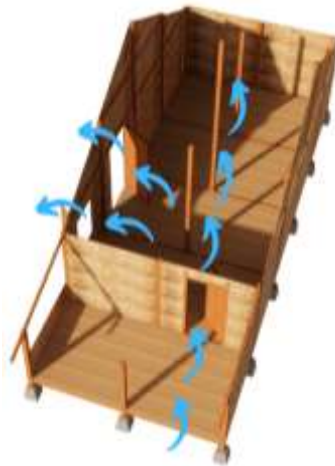
Figure 17: Airflow in Sulah Nyanda House (Source: Personal Document, 2024)
