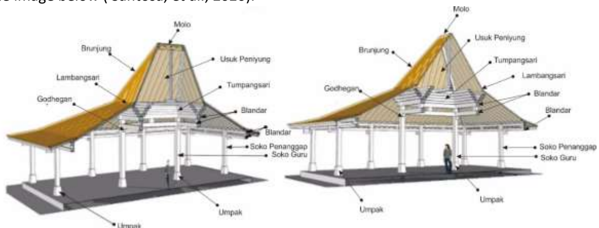
Figure 9. Elements of a Joglo House Source: Sketch 2024
