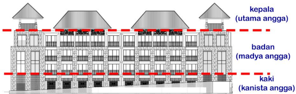
Figure 12 Application of the 3 Tri Angga hierarchies on the building facade (source: image by the author)
