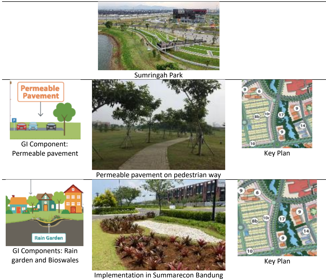
Figure 6. Open space with rain garden and water-absorbing bioswales (Source: Observation, 2024)
