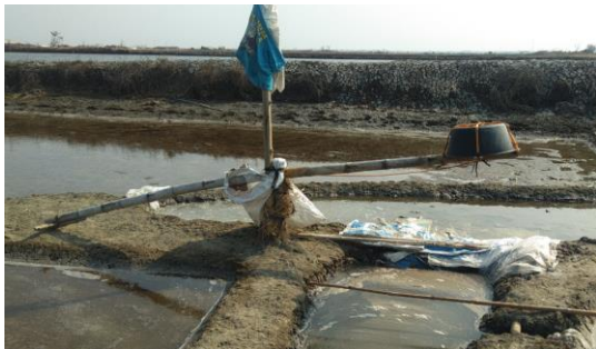
Figure 3 “Ebor” as a traditional tool that is used to move water into salt fields
