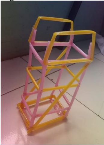
Figure 7 Student earthquake resistant building prototype
