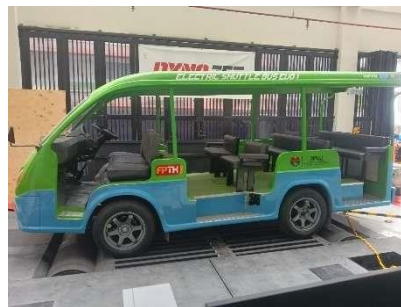
Gambar 1. Pengujian Dynotest Electric Shuttle Bus
