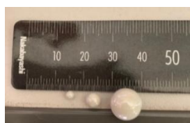
Figure 2. The different sizes of Zirconium balls used in the milling process
